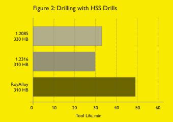
Figure 2: When drilling, the cutting speed can be increased up to 40% with the same tool life of the drill, 1000 mm.
