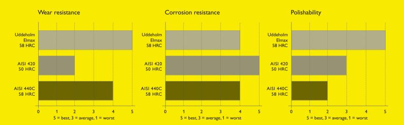
Relative property profile for Uddeholm Elmax, AISI 420 and AISI 440C in plastic moulds.
