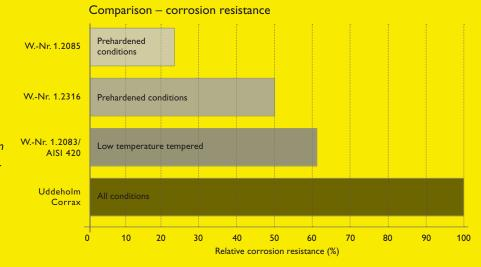
Uddeholm Corrax has very good corrosion resistance, better than the corrosion resistance of standard grades used for plastic moulding. The corrosion resistance is the same in all heat-treated conditions.
