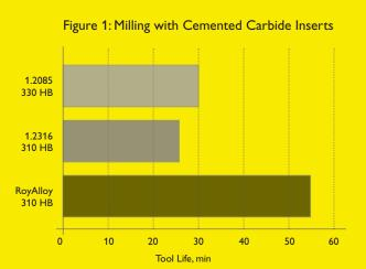
Figure 1: During cavity milling the tool life is almost double when cutting with the same speed, 270 m/min. Alternatively, the cutting speed can be increased considerably with the same tool life as with 1.2085.
